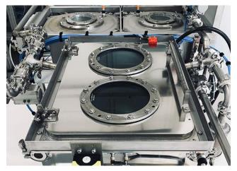
PPC - Pulsated Pressure Cleaning: Two modes of action for significantly improved component cleaning
